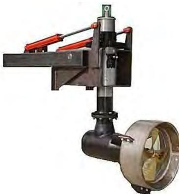
These thrusters can turn 360° and be leveled upwards when not in use. The most sophisticated steering system is when the thrusters are connected to a GPS system and linked to the route coordinates. (Dynamic Positioning System). In any case a GPS system is useful. It will monitor the position of laid cables.
